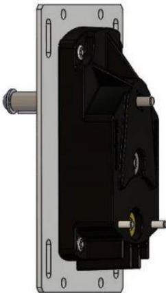
**Step 8:** Attach the ToughBox Micros with 1/4-20x1000 Thread forming screws (am- 1182). Do this to both sides of the chassis.
